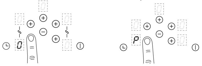
For quick operation, touch the minus key for quicker access to the Power Boost level.
